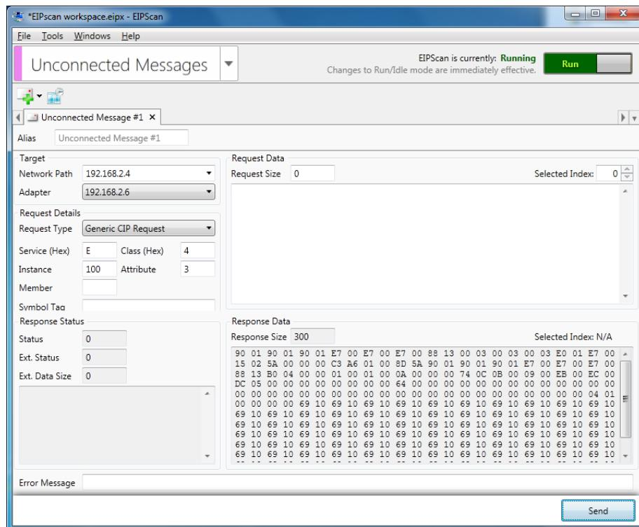
Example 2: Reading the power supply data (voltage on terminals 1 and 2) of a Multi-line 2 unit:
