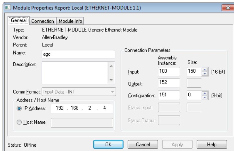
Input assembly instance must be 100 with a size of 150 words or 300 bytes.
