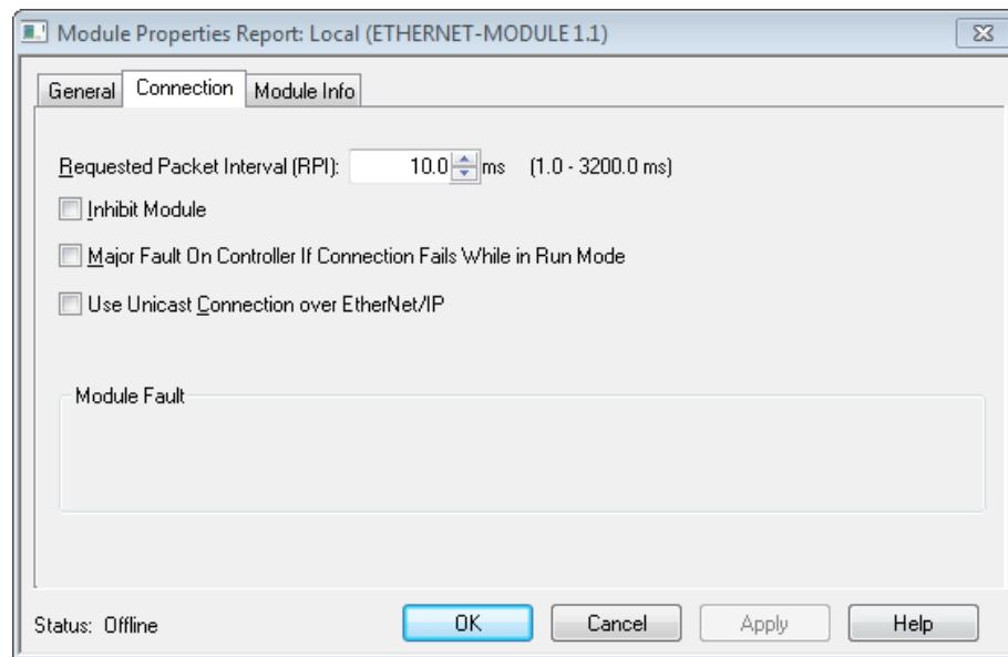
You can tick “Use Unicast Connection over Ethernet/IP” or leave it unticked. The RPI delay should not be lower than 10 ms.
