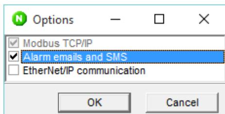
The Ethernet/IP communication will be up and running after a short reboot of the option N card;
