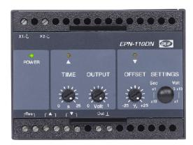
The potentiometer converts the relay output of a PI step controller to a control voltage for the speed governor/AVR, including DEIF's load sharing unit type LSU, DEIF's synchronisers type FAS, or any other type of PI step controller with relay.
