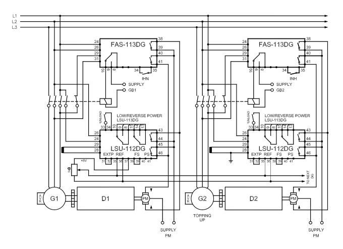
Application for mechanical governors synchronisation and fixed load to busbar with load sharing. No frequency control.
