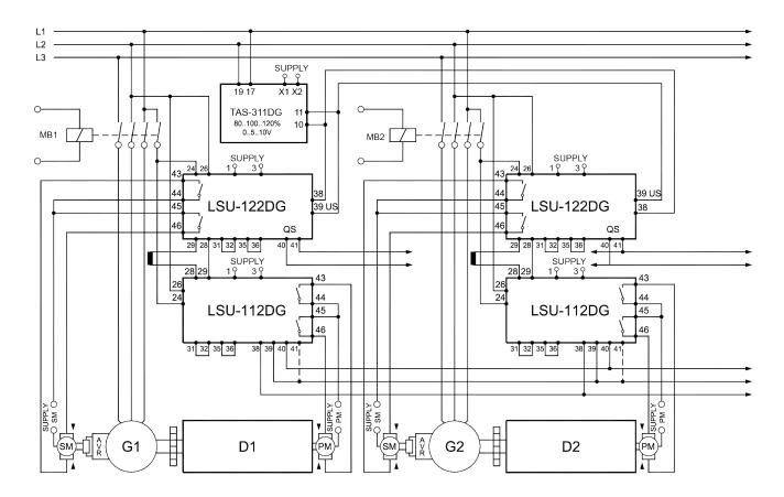
Application for mechanical governors and motor potentiometer controlled AVRs. Normal active load sharing. Normal reactive load sharing.
