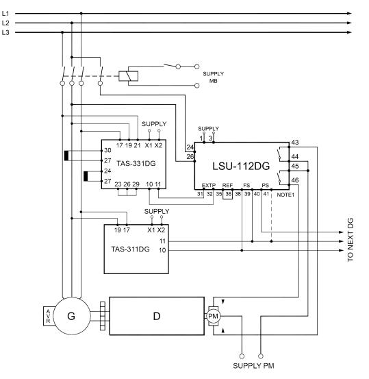
Note 1: Terminals 39 + 41 are internally connected.
