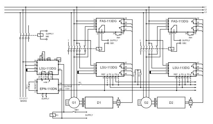
Application for mechanical governors synchronisation and mains peak lopping (no frequency control) island load sharing (with frequency control).
