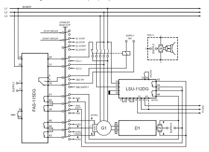
Note 1: Terminals 39 + 41 on the LSU-112DG are internally connected.
