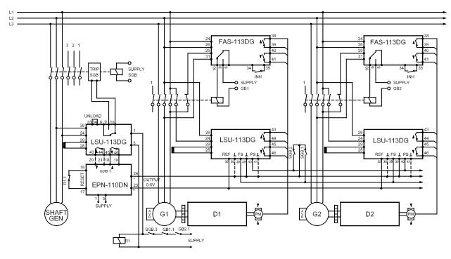
Application for synchronisation of a shaft generator to a generator set with load transfer.
