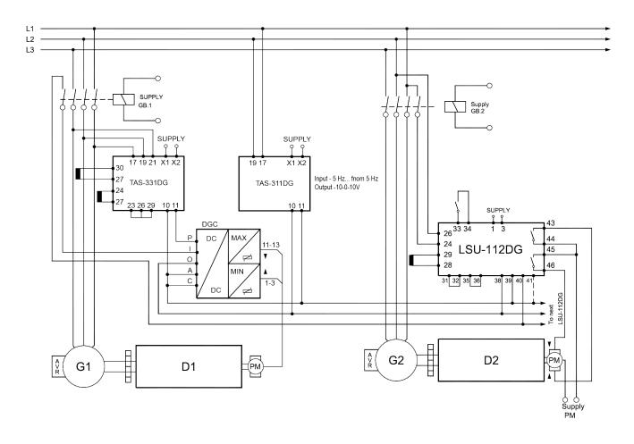
Normal load sharing using the DGC-ITF (ITB) together with the LSU-112DG.
