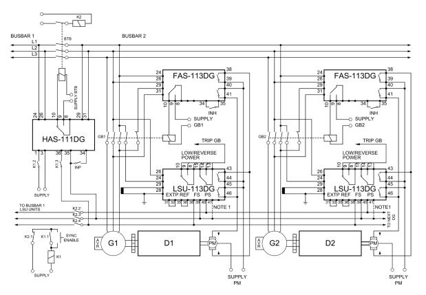
Note 1: Terminals 36 + 39 + 41 on the LSU-113DG are internally connected.
