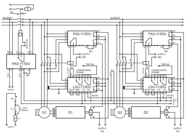
*Note 1: Terminals* 36 + 39 + 41 *on the LSU-113DG are internally connected.* Application for synchronisation of a bus tie breaker with unload of generators and tripping of breakers.
