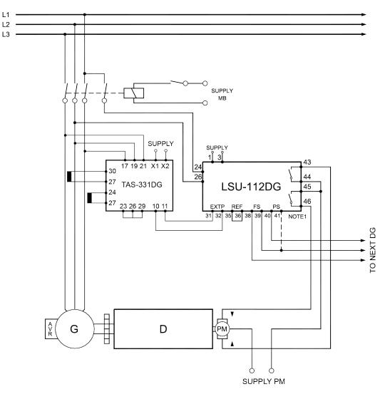
Note 1: Terminals 39 + 41 are internally connected.
