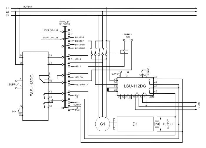
Note 1: Terminals 39 + 41 on the LSU-112DG are internally connected.
