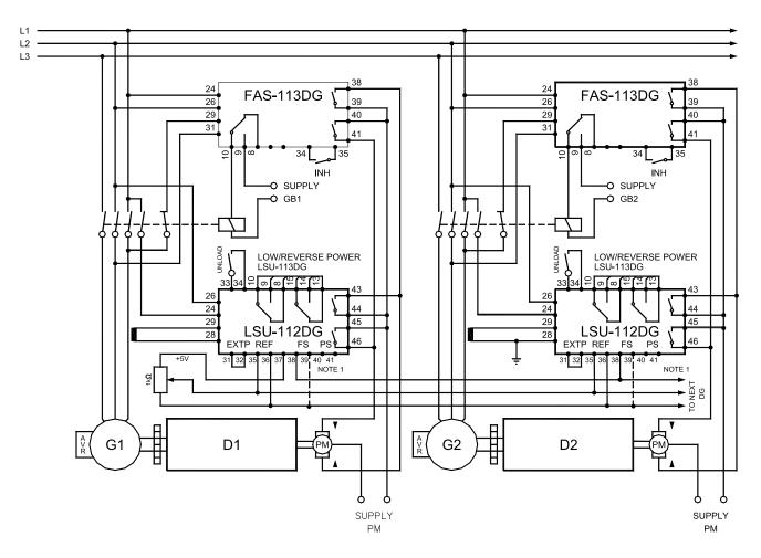
Note 1: Terminals 36 + 39 on the LSU-112DG are internally connected.
