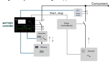
The iE 150 Marine Battery controller can support the load, so that the genset can run at its optimal load point.
