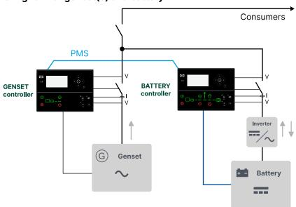
To improve power quality, the controller can supply peak loads while gensets start. The controller can support the load, so that the genset can run at its optimal load point. If the ESS is designed to supply the busbar load, the ESS can be the only source connected to the busbar.
