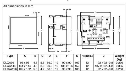
The instrument is mounted by means of the 2 fixing elements. For instruments with IP54 or IP66 protection, use all 4 fixing elements and the rubber gasket (included in the packing).
