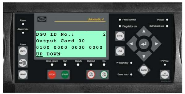
Binary input for channel 0 is indicated as the first digit seen from the left. A low status is indicated with a 0, a high status is indicated as 1. If the input channel is selected for analogue, it is indicated with an A.
