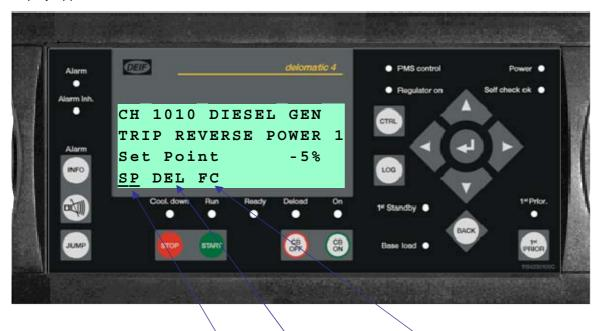
Each protection has a setpoint (SP), timer (DEL) and a Fail class(FC) that can be configured within defined limits. All parameters are password-protected to prevent unauthorised personnel from changing the settings.
