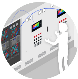
Base-mounted with display Mount the controller at the base and the display located further away.
