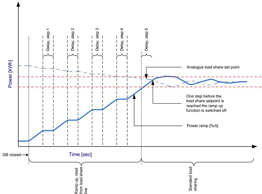
When menu 2614 is enabled, the power setpoint continues to rise in ramp up steps, determined by menu 2615, towards the load sharing setpoint. The delay time between each ramp up step will be determined by menu 2613. The ramp up will continue until the load sharing setpoint is reached, and then the regulator will be switched to standard load sharing mode.
