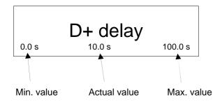
Parameter example: D+ delay setting. Use ▲ or ▼ to scroll through the settings list. If change of settings is necessary, press ← and enter the password. Then use ▲ or ▼ to change values. Use ESC to leave settings.
