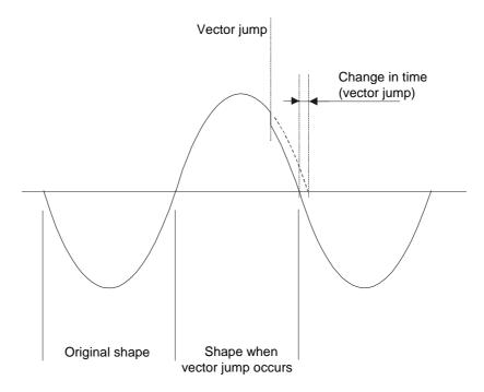
Again, comparing the half-sine curve time duration with the previous ones, a sudden change in time can be detected. This is the vector jump.
