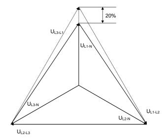
Phase-neutral or phase-phase, both the generator protections and the busbar/mains protections use the selected voltage.
