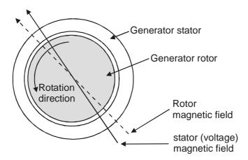
If a mains failure occurs, the time lack of the stator magnetic field (and the output voltage) will change (jump). This is called a vector jump.
