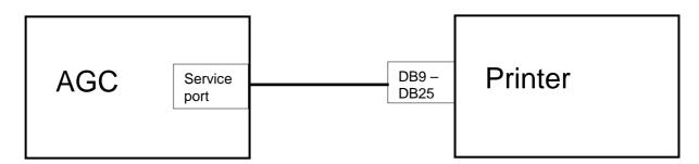
The cable used between the controller unit and the printer is a 9-pole null-modem cabel. This cable is also used for the connection between the PC and the unit, if the PC utility software is used for configuration.
