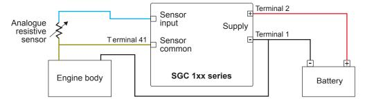
\*SCP connections for Analogue input 2 used as Fuel level sensor with the reference configured as Battery Negative
