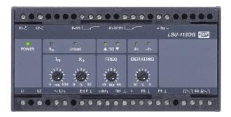
DEIF's Uni-line Load Sharing Unit, the LSU-113DG, provides load sharing with reverse power protection and low power detection between generators and interfaces to a governor through an electronic potentiometer (EPQ96-2 or EPN-110DN).
