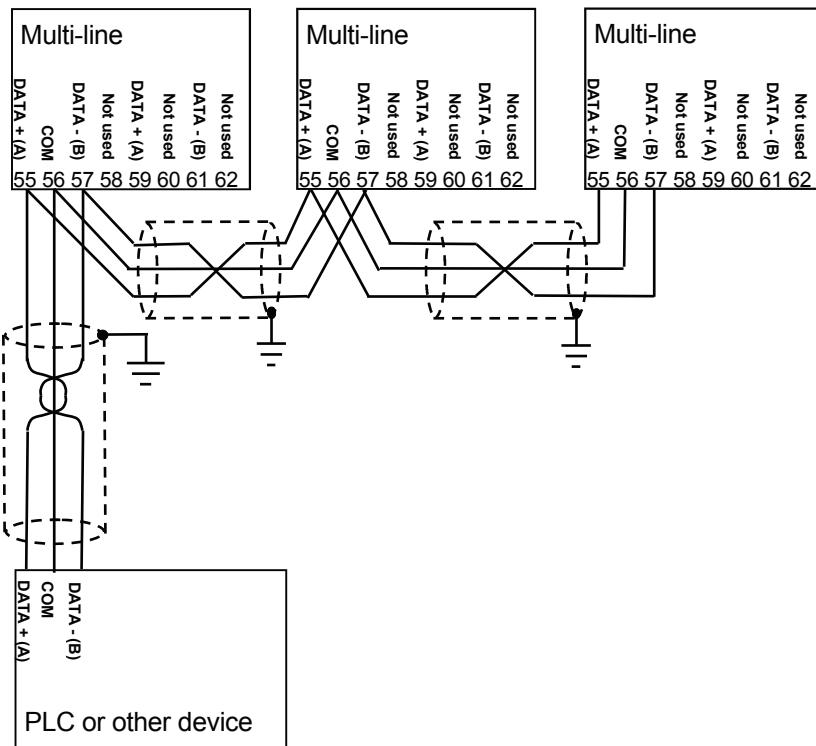
**⚠** This solution is only feasible if the COM line is insulated. Check PLC/other device before connecting.
