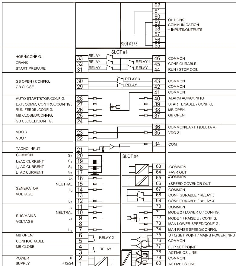
The terminal 36 must be connected depending on the hardware type of the BGC.
