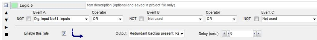
This line is also used in both controllers to indicate that a backup controller is present in application supervision.
