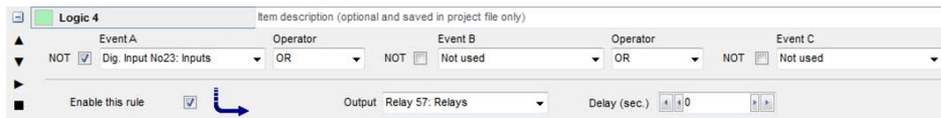
Both controllers will have this line saying that if input 23 is **not** active and thus is the controller that has control, it sets the opposite controller in redundant mode with output 57. One of the controllers will need a small delay on relay output 57 to avoid timing issues when both controllers are powered up at the same time.
