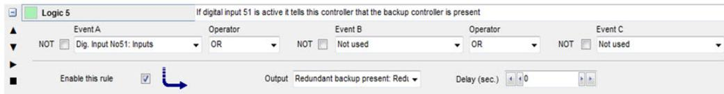
This line is used in application supervision to indicate that a backup unit is present.
