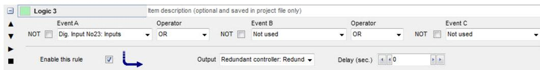
Both controllers will have this line saying that if input 23 is active, then this controller is redundant. When both controllers are powered up at the same time, it would be the first one ready that will set the opposite controller to be redundant.
