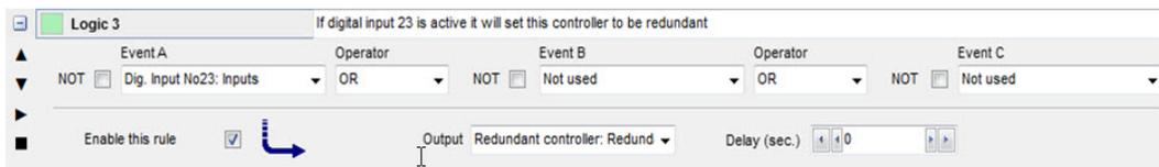
When the preferred controller is fully operational, this input is activated to hold the redundant controller in standby mode.
