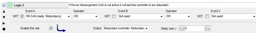
The line above keeps the preferred controller in standby mode when powering up, to prepare the CAN communication, and does not interrupt control of the redundant unit until the preferred controller is ready for operation.
