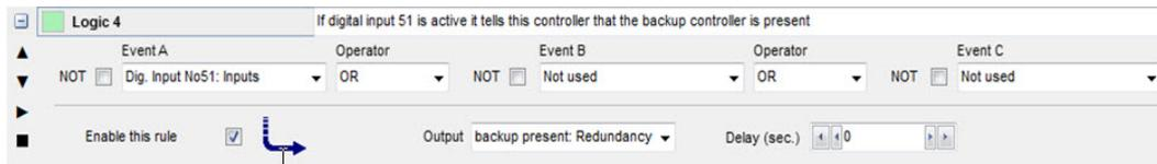
This line is used in application supervision to indicate that a backup unit is present.
