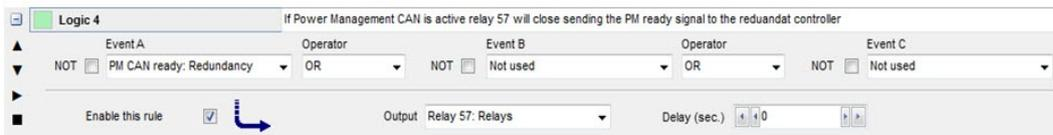
When power management CAN is ready for operation, the preferred controller requests control, putting the redundant unit in standby mode.
