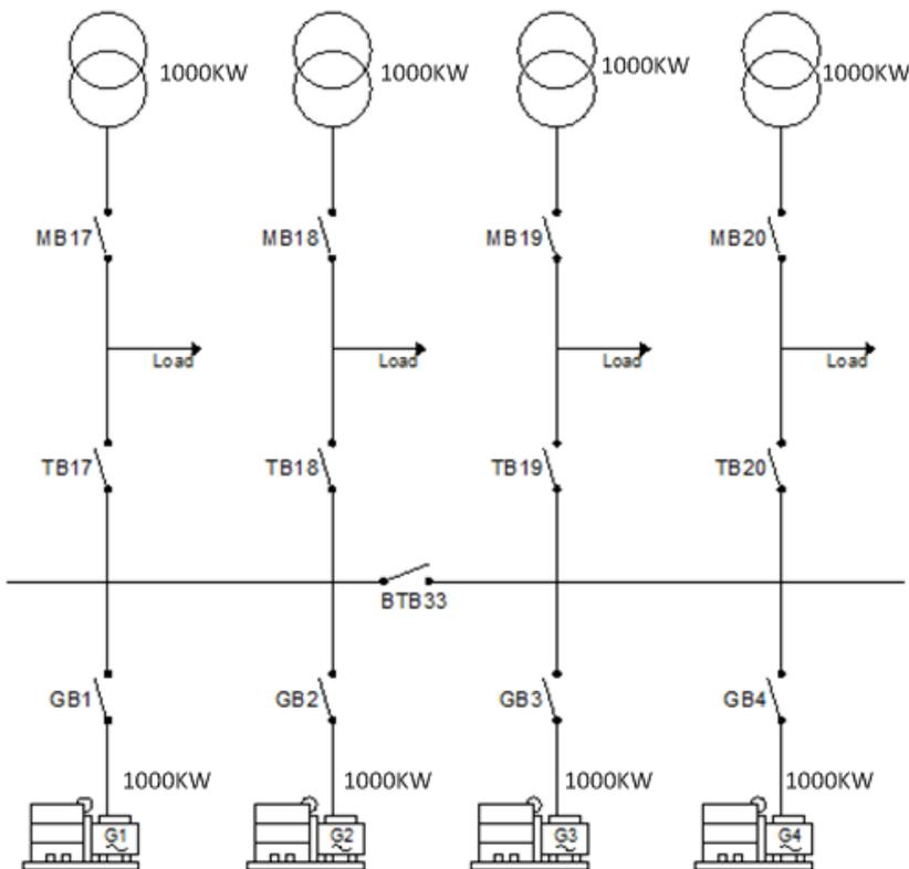
The nominal power values of each mains or DG unit are used in the calculation. This means that its static nominal power values are used for the short-circuit limitation calculation.
