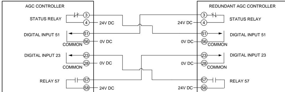
**i** Relays and digital inputs for this function must be placed within this terminal range: 1-28 or 43-64.
