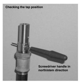
A screwdriver can be used as a pointer to make sure that the position of the tap is correct according to the ship's stem (on land-based installations according to north).
