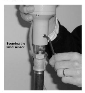
Tighten the wind sensor on the tap.
