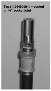
In the above illustrations a  $\frac{3}{4}$ " water pipe and a  $\frac{3}{4}$ " socket joint are used as support for the tap for the wind sensor. It is recommended to use a washer between the  $\frac{3}{4}$ " socket joint and the tap to obtain a good joint.
