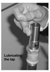
The tap is lubricated with copper grease. This is necessary to enable demounting of the wind sensor for service.
