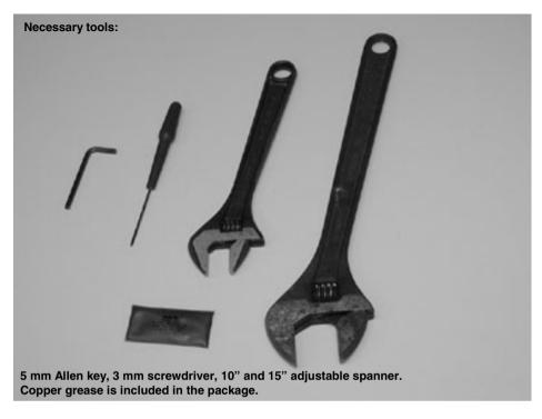
Necessary tools. Other types can be used, e.g. 20 mm and 36 mm fixed spanners.
