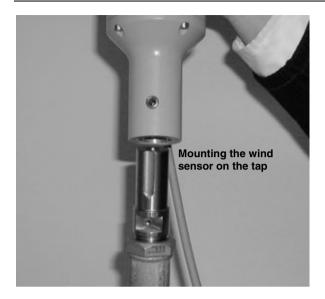
The wind sensor is mounted on the tap as illustrated. Notice that the "key way" on the tap (screw on the wind sensor) must point at the ship's stem, or north on land-based installations.
