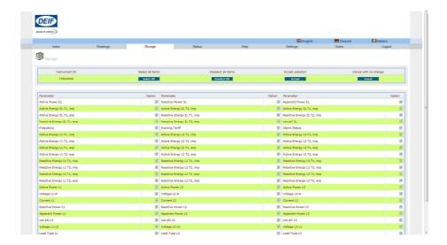
In this page, for every item in the readings page, a checkbox allows to include or not this parameter in the stored data.
