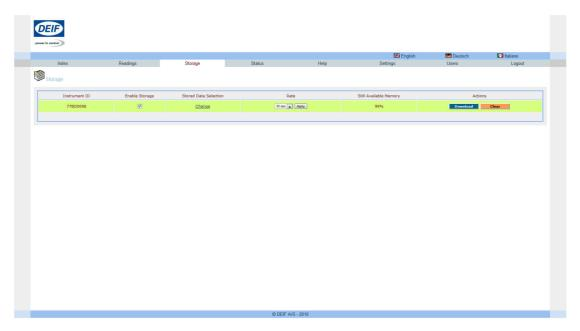
You can enable the storage of data read from the instrument selecting the Enable Storage checkbox to begin the process. The sampling rate can be changed selecting the proper rate and pushing the **Apply** button.
