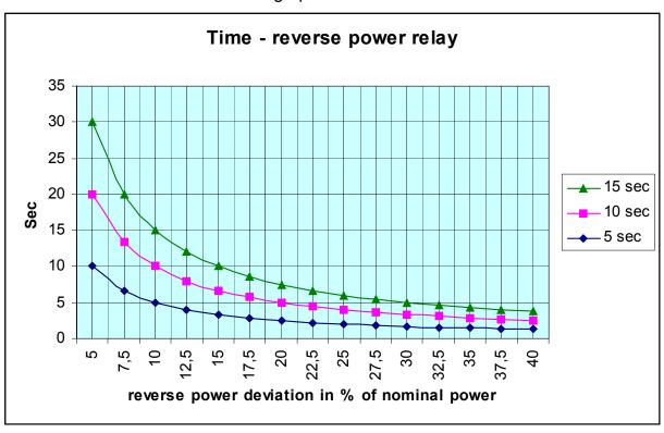
If the –P set point is exceeded by 10% of nominal power, the inverse timer functionality gives the same delay as the time potentiometer. If the –P set point is exceeded by 20% of nominal power, the delay will be half the value set on the time potentiometer.
