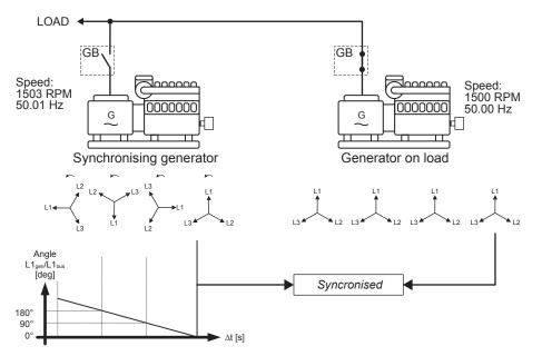
In this example, the synchronising genset is running at 1503 RPM  $\sim$  50.1 Hz. The generator on load is running at 1500 RPM  $\sim$  50.0 Hz. This gives the synchronising genset a positive slip frequency of 0.1 Hz.
