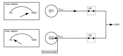
The illustration shows that at a given negative slip frequency, the incoming genset will *receive* power from the original genset (reverse power).
