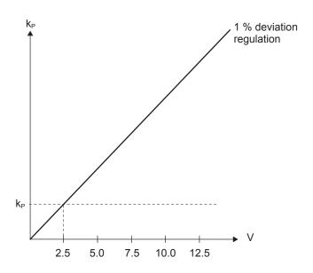
A 1 % regulation deviation occurs. With the Kp setting adjusted, the deviation causes the output to change 2.5 V. The table shows that the output of the AGC changes relatively much if the maximum speed range is low.
