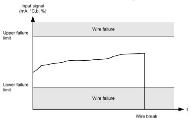
Configure the parameters for Wire break under **Settings > I/O settings > Inputs > Multi input > Wire fail #**, where # is 20, 21, 22 or 23.
