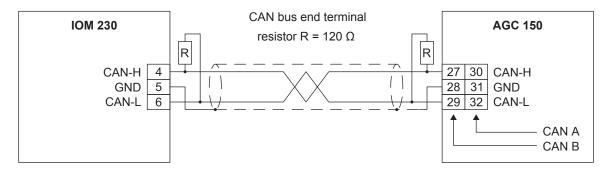
The cable shield must not be connected to ground, only to the GND terminals.
