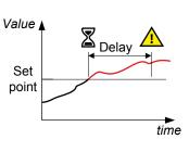
Configure the parameters under Settings > Generator > Current protections > Over-current > I> #, where # is 1 or 4.
