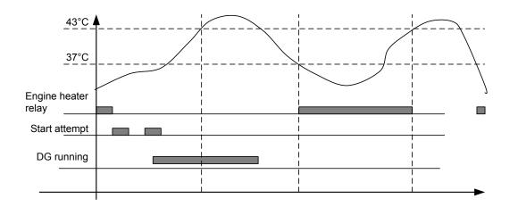
The engine heater contains a set point and a hysteresis. In the example, the set point is 40 °C with a hysteresis of 3 °C. The AGC 150 will open the engine heater relay when the engine has reached 43 °C, and close when the engine temperature is 37 °C.
