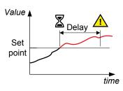
The alarm response is based on the highest phase current true RMS value, with the direction from the active power from the source, as measured by the controller.
