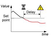
Configure the parameters for Busbar under-voltage under **Settings > Busbar > Voltage protections > Under-voltage > BB U< #**, where *#* is 1 to 4.
