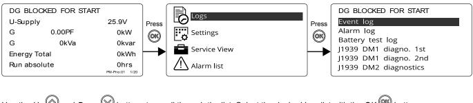
Use the  $Up \bigotimes$  and  $Down \bigotimes$  buttons to scroll through the list. Select the desired Log list with the  $OK \bigotimes$  button.
