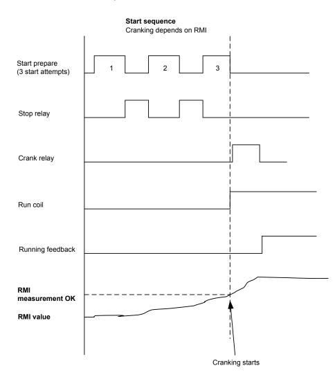
The crank/start is initiated as soon as the Start threshold limit is reached. By default, the AGC 150 waits until the Start prepare timer has expired and the Start threshold conditions are reached before the crank relay/start is initiated. This can be changed from parameter 6185, where the Start prepare type can be changed to Interrupt start prepare, which means that it is allowed to interrupt the start prepare and initiate as soon as the Start threshold conditions are reached.
