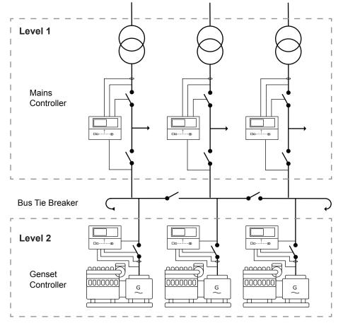
When setting up the phase sequence alarms, it can be helpful to activate MB fail start in some of the mains controllers.
