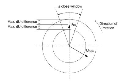
The pulse is issued in accordance with the settings for static synchronisation, depending on whether the GB or the MB is to be synchronised.
