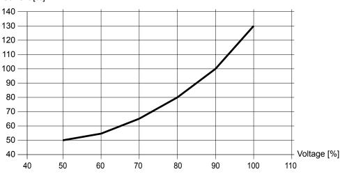
When the actual values represent a point above the curve, the breaker is tripped. The curve shows that the generator breaker will trip when the generator voltage is below 50 % of rated, and the current is above 50 % of rated.
