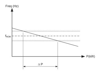
This can be used if the generator must operate as a peak load machine.
