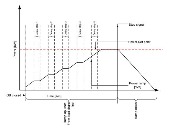
When *Island ramp* is enabled, the power set point continues to rise in ramp up steps towards the load sharing set point. The ramp up will continue until the load sharing set point is reached and then switch the regulator to standard load sharing mode.
