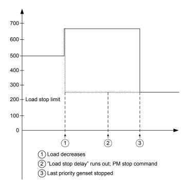
**NOTE** If the priority order is changed, but does not seem to change as expected, it is because the load-dependent stop function is not able to stop the lowest priority after having started the new first priority. That would cause two DGs to be running at low load instead of one DG.
