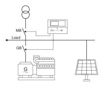
In Peak shaving mode, the PV inverters attempt to take all the load. As long as the load is below the Peak shaving set points, the genset is stopped. When the load increases above the Peak shaving set point, the genset starts.
