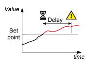
Configure the parameters under Settings > Busbar > Frequency protections > Over-frequency > BB f> #, where # is 1 to 3.
