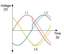
Configure the parameters for Vector jump under Settings > Busbar > Additional protections > Vector shift.
