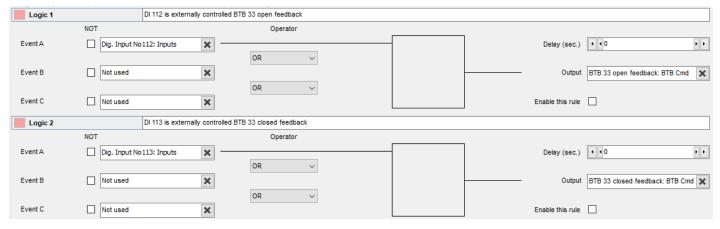
The power management system monitors the external controlled BTB feedbacks and responds to changes in the breaker position. For example, when the BTB is opened, power management detects that there are new busbar sections.
