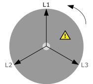
Configure the parameters under Settings > Generator > Current protections > Negative seq. current > Negative. seq. I.
