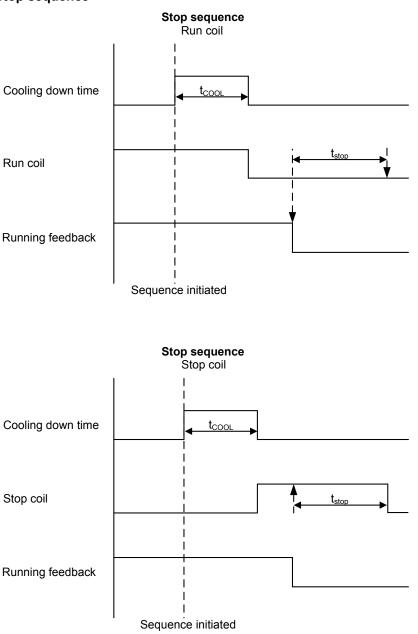
The Stop sequence will be activated if a stop command is given. The Stop sequence includes the cooling down time if the stop is a normal or controlled stop.
