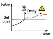
Configure the parameters under Settings > Generator > Frequency protections > Over-frequency > G f> #, where # is 1 to 3.
