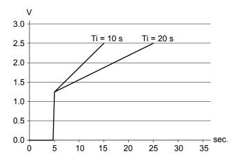
The output reaches 5 mA twice as fast at a Ti setting of 10 s than with a setting of 20 s.
