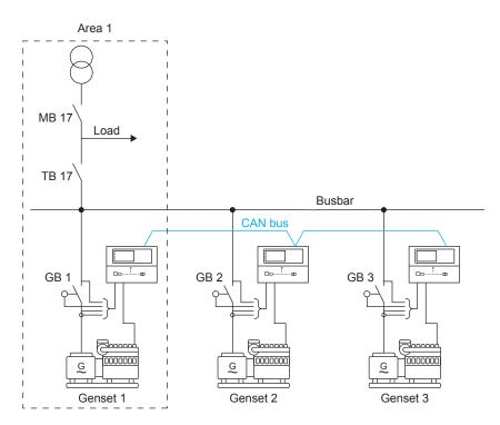
A tie breaker in the mains controller can be operated in an island application. The Power capacity set point (parameter 8192) is used to ensure that the generators produce enough power to take the load. This protects the generators from going into overload.
