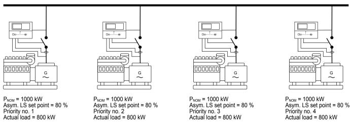
When the load is increasing or decreasing, the genset with the last priority will take the deviations, so the other(s) can be kept at a more optimum load point. If the load should exceed 3200 kW in the example above, the load will be shared equally between them. If the load afterwards decreases to a level below 3200 kW again, the three first gensets will regulate towards the 80 % again, and the last will take the deviations.
