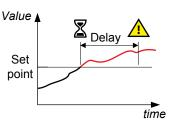
Configure the parameters under Settings > Generator > Power protections > Overload > P> #, where # is 1 to 5.
