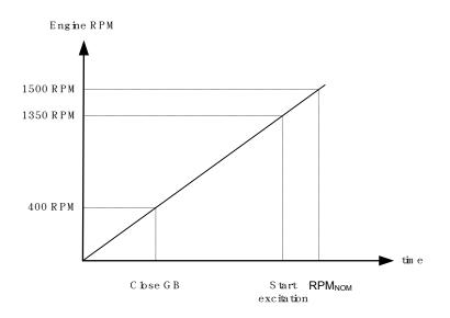
The diagram above shows that the GB will be closed at 400 RPM. When the engine RPM has reached the set point (1350 RPM), the excitation is switched on.
