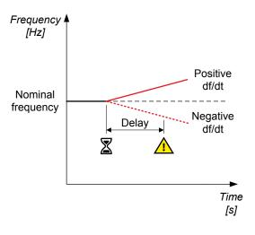
Configure the parameters for ROCOF df/dt under Settings > Busbar > Additional protections > df/dt (ROCOF).
