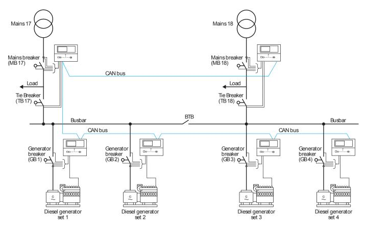
NOTE The diagram shows four generators, but the system supports up to 32 connected genset or mains controllers.
