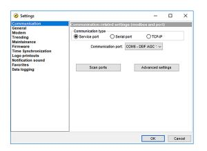
Select the *TCP-IP* button to enter the IP address. Press the *Test* button to check if the connection is successful, then press the *OK* button.
