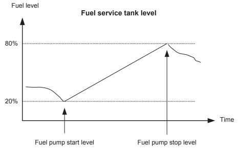
The fuel pump starts when the level reaches 20 % and stops again when the level has reached 80 %.
