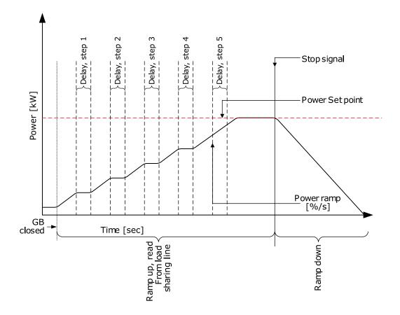
Configure the Power ramp up function under Settings > Power set points > Loading/Deloading ramps > kW ramp up speed.
