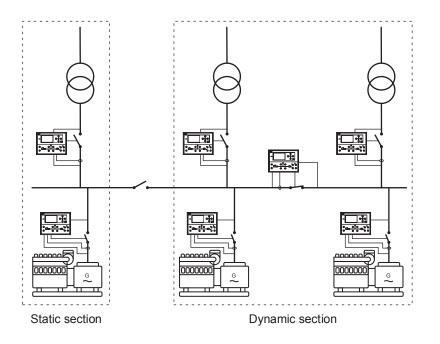
**Static section**: This part of the application can not be divided further by BTBs. If there are no BTBs in the application, the whole application will be a static section.
