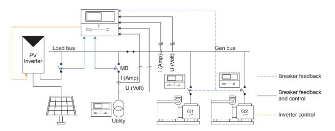
**NOTE** The AGC 150 is still measuring the total generator output.
