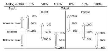
100 % offset is commonly used with inverse output, like in the previous cooling example.
