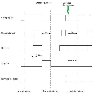
Run coil can be activated from 0 to 600 s before crank (starter) is executed. In this example, the timer is set to 1.0 s.
