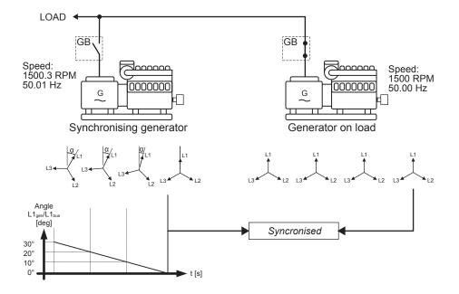
The frequency controller uses the angle difference between the generator system and the busbar system as control parameter. This is illustrated in the example above, where the phase controller brings the phase angle from 30 to 0 $^{\circ}$ .
