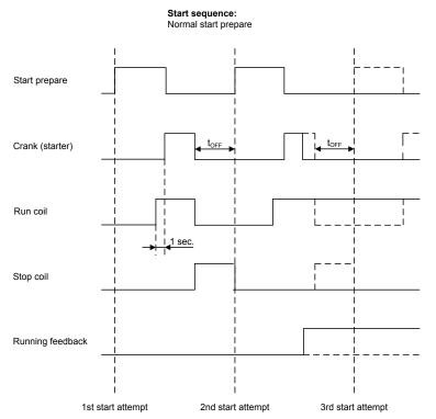
In this example, the Run coil opens between the start attempts. This is because the Run coil type is set to pulse. When the engine gets running detection, the run coil will be kept closed until the stop sequence is initiated. If the Run coil type has been set to Continuous, the run coil will be kept closed between the start attempts until start failure, or the stop sequence opens it.
