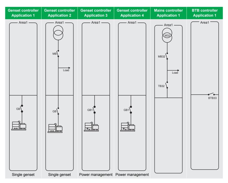
The pre-configured standard applications can be chosen directly from the controller under **Settings > Basic settings > Application type > Standalone or PM > Application select**.
