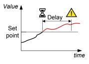
Configure the parameters under Settings > Generator > Current protections > Unbalance current > Unbalance I #, where # is 1 or 2.
