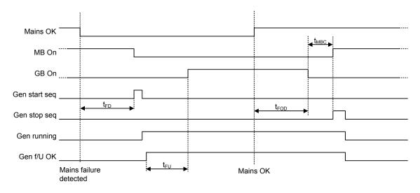
Figure 5.5 Example 2: Mains fail control (Start engine)
