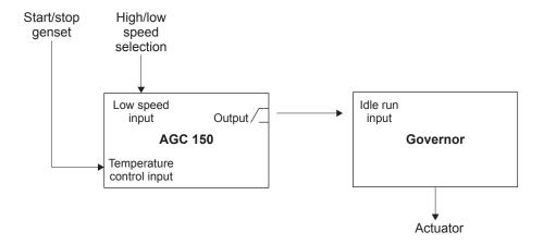
When the function is enabled, two digital inputs are used for control purposes:
