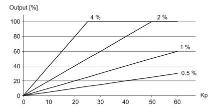
In this example, we have a 2 % regulation deviation and an adjusted value of the Kp = 20. The calculated regulator value of the controller is 40 %. Now the pulse length can be calculated with a period time = 2500 ms:
