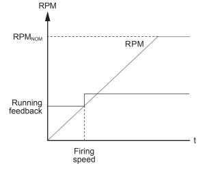
The diagram illustrates how the digital running feedback is activated when the engine has reached its firing speed.
