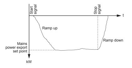
**NOTE** The set point of the mains power export can be adjusted to 0 kW. This means that the genset will be parallel to the mains but no power import or export.
