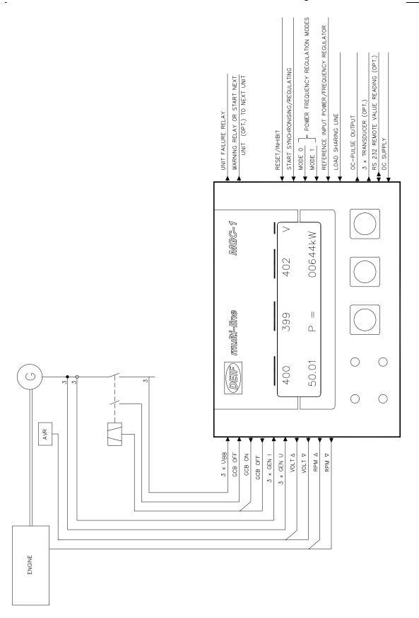
A principle diagram of connecting MGC-1 is shown above.
