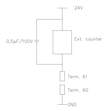
A 0.5μF (≥100V) capacitor should be connected in parallel with the energy counter.
