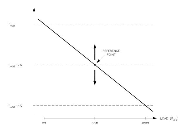
A smaller speed droop range than the recommended 4%, may result in a fast (may be too fast) dynamic control loop and thus an unstable power plant. A larger speed droop range than the recommended 4%, may result in a slow (may be too slow) dynamic control loop.
