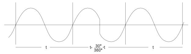
The vector jump is detected by comparing the measured period length  $t_N$  with a mean of earlier period lengths. The difference in period length is expressed in degrees with respect
