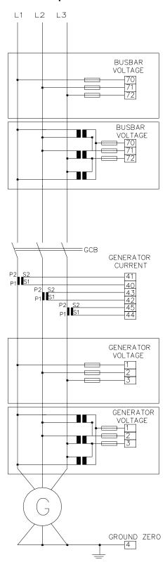
When ordering a MGC-1 the correct range of AC-inputs must be specified. It is possible to set current and voltage trafo specifications in the display.
