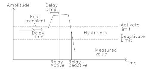
The protective relays can be programmed either to be self-resetting when a fault disappears (shown above) or holding the output signal until the fault is acknowledged through push-button or external acknowledge signal.
