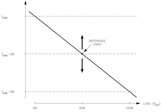
The graph shown above is controlled by three parameters.  $f_{NOM}$  the nominal power and the speed droop (set as % of  $f_{NOM}$ , here 4%). If the frequency controller uses an external source the graph will also change with the external source. E.g. if the analog set-points are set to  $0mA \approx 45Hz$  and  $20mA \approx 55Hz$ , the  $f_{NOM}$  at the y-axis is 47Hz at 4mA. All other regulator
