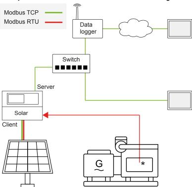
The controller can communicate over Modbus as the client and/or server device. The controller can communicate with the PV system using Modbus TCP or Modbus RTU. The controller reads from power meters or genset controllers using Modbus RTU.
