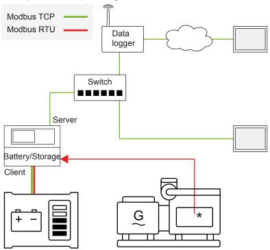
The controller can communicate over Modbus as the client and/or server device. The controller can communicate with the ESS using Modbus TCP and/or Modbus RTU. \* The controller reads from power meters or genset controllers using Modbus RTU.
