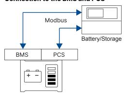
Select **DEIF Generic** in *ESS protocol* (parameter 7561) to control the PCS and select **DEIF Generic** in *BMS protocol* (parameter 7682) to control the BMS.
