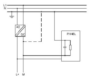
All the electronic devices in the control system must be properly grounded. Grounding must be performed according to applicable regulations.
