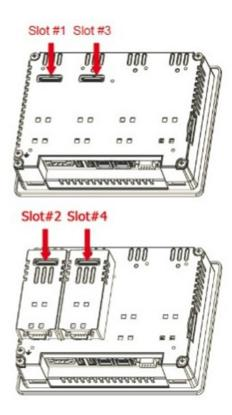
Slot #2 and slot #4 are available only if the plug-in module has a "bus extension connector".
