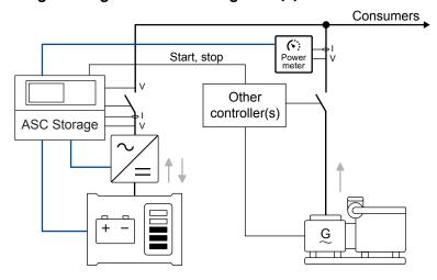
The ASC 150 Storage controller can support the load, so that the genset can run at its optimal load point.
