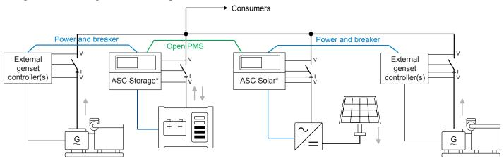
**NOTE** \* You can use multiple controllers in the application. Power measurements can be connected to the closest ASC controller.
