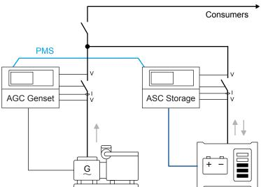
To improve power quality, the ASC 150 Storage can supply peak loads while gensets start. The ASC 150 Storage controller can support the load, so that the genset can run at its optimal load point. If the ESS is designed to supply the busbar load, the ESS can be the only source connected to the busbar.
