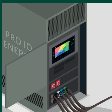
Front mounted controller with combined display
