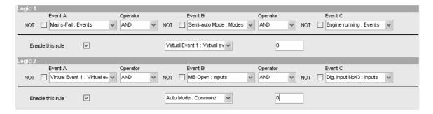
In this example the unit automatically goes to auto mode when these conditions are met:
