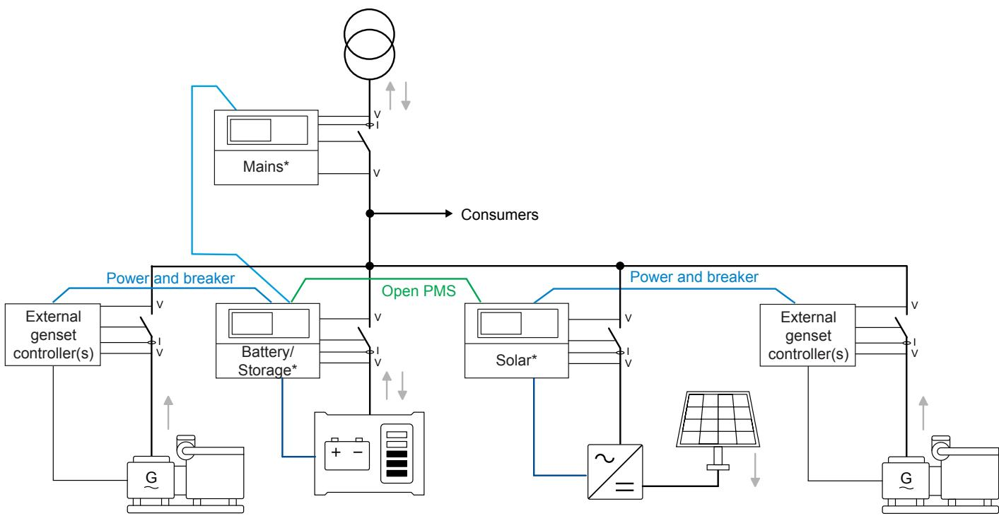
**NOTE** \* You can use multiple controllers in the application. Power measurements can be connected to the closest battery/storage or solar controller.
