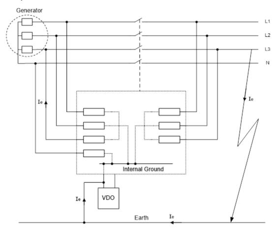
The neutral and generated neutral for the three voltage measurements are connected to the internal ground. If there is a ground connection (in this example, the VDO) the internal ground is connected directly to earth, without any galvanic separation.
