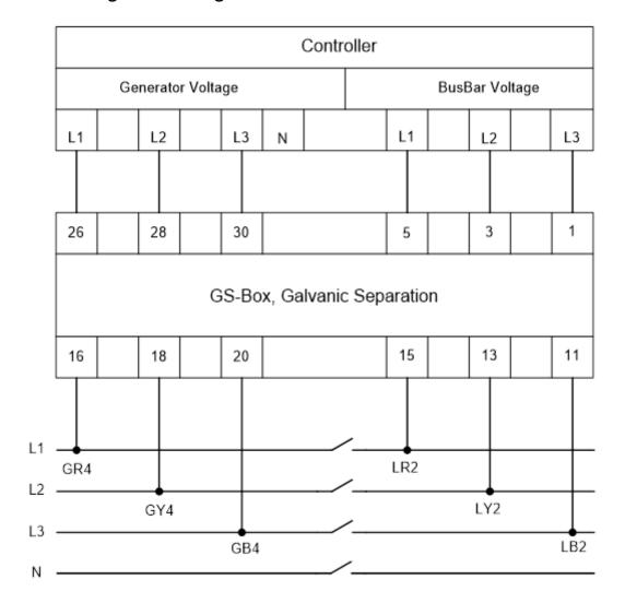
**NOTE** If you have earth problems, to avoid interruption from earth faults, you must remove the generator voltage neutral connection from the controller.
