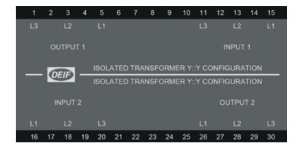
**NOTE** The GS-box uses transformers to transfer the input voltages to an identical set of output voltages. The voltage range for the 440 V AC version is 380 to 480 V AC.
