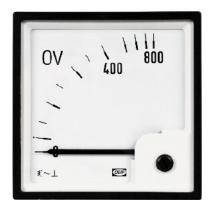
The zero voltage meter type NEQ is a moving iron instrument calibrated to full scale deflection at twice the nominal mains voltage, whereas 2/3 deflection corresponds to nominal mains voltage.
