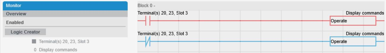
In this example, a **GENSET** controller has a digital input associated with an OPERATE block for the function *Display commands*. The value set in the OPERATE block relates to value for the command source.
