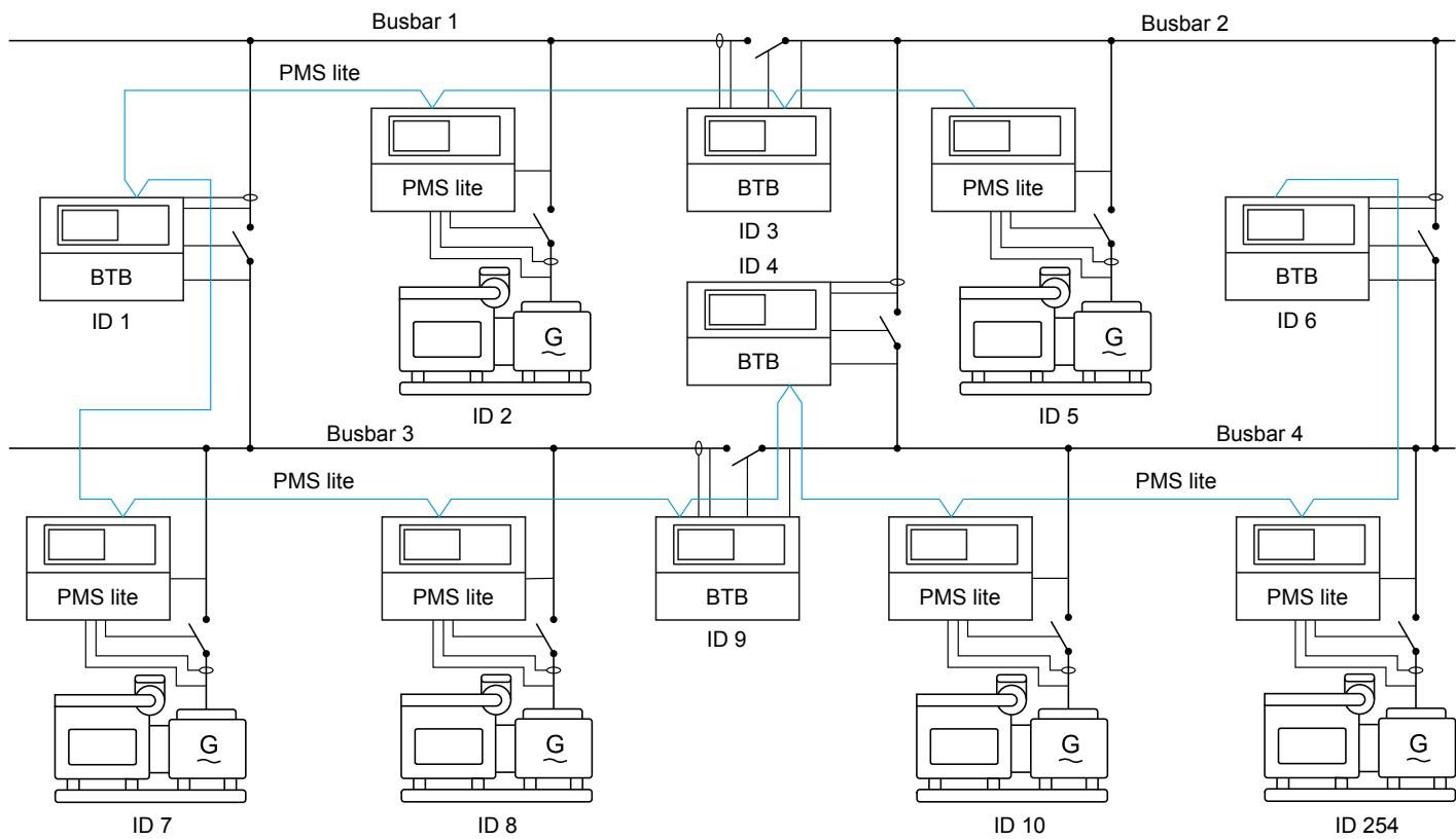
**NOTE** To control gensets in a standard power management system, use iE 150 Generator or AGC 150 Generator controllers.
