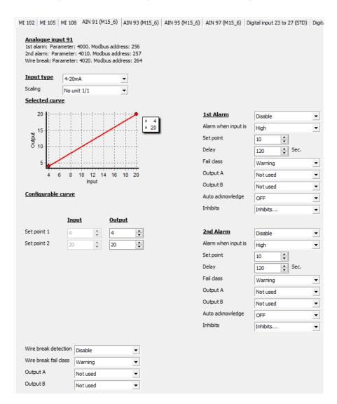
**Configure the curve**: Select the *Output* values for *Set point 1* and *Set point 2*. For an inverse proportional curve, *Set point 1* has the higher output value.
