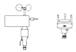
Remove the tap for the old sensor 879.3c and mount the new sensor. Notice that the tap is fixed on the new sensor and is not to be removed.
