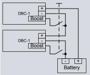
5 A + 5 A = 10 A DC Possible 5 A + 10 A = 15 A DC Possible 10 A + 10 A = 20 A DC Possible
