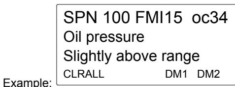
The alarm log always shows the DM1 (active alarms) as default. By selecting DM2 (move the cursor under DM2 and press ENTER), the historical alarm list can be shown.
