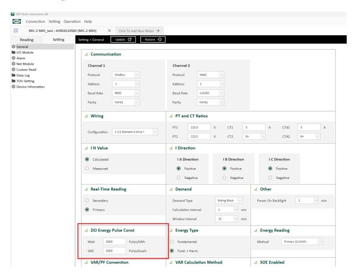
Once you have calculated the pulse constant, you can configure the pulse constant setting from the display, with Modbus, or using the utility software.
