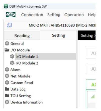
2. From the Al Setting section, you can configure the Al type. The default type is voltage, where you can configure the input as 0 to 5 V or 1 to 5 V.
