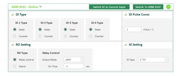
3. To see the current AI types, you need to click the Switch AI to Current Input button Switch AI to Current Input Switch AI to Current Input
