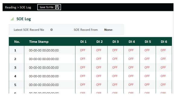
The SOE begins to record immediately when the MIC-2 MKII is powered on. The data is not lost in the event of a power outage or a shutdown. If you change the I/O module in which the SOE function is configured, the SOE records are lost.
