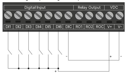
V DC is the supply for the digital inputs.
