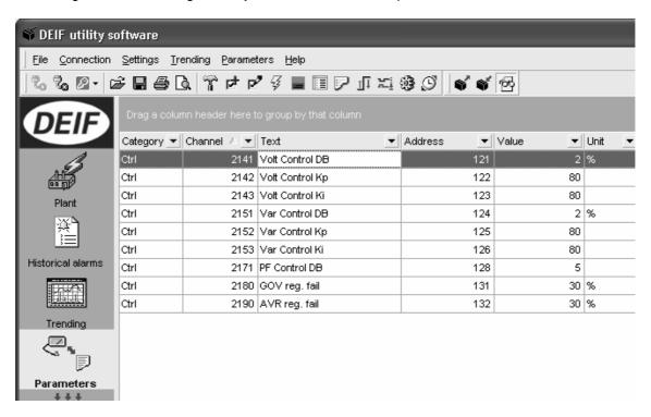
The screen dump above illustrates the controller settings of the voltage and var controller. As an initial setting before the first start up, the  $K_P$  and  $K_I$  of the voltage and var controllers are set to a low value.
