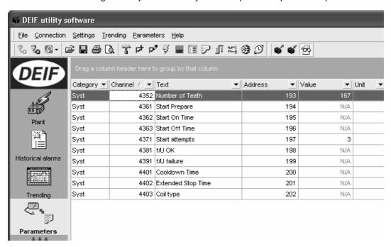
In the screen dump above, the adjustments for the start and stop sequences are illustrated. Since the function control settings include parameters for the entire functionality of the multi-line 2, they
