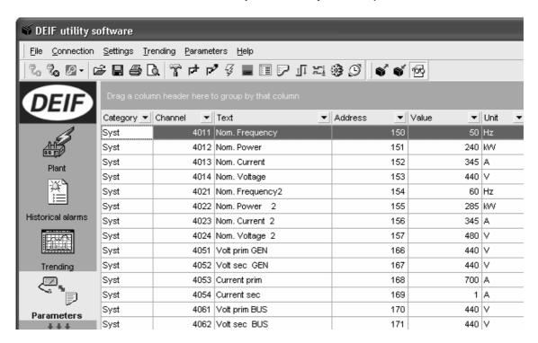
In the PC utility software it is presented as illustrated on the screen dump above. The correct values are supplied by the switchboard manufacturer.
