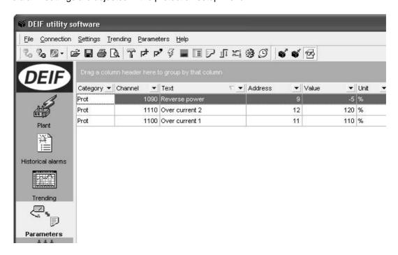
In the PC utility software it is presented as illustrated on the screen dump above or similar. The screen dump includes the protection alarms of the standard multi-line 2. The number of alarms depends on the options selection of the individual unit. The actual alarm parameters are adjusted according to customer requirements and application requirements.
